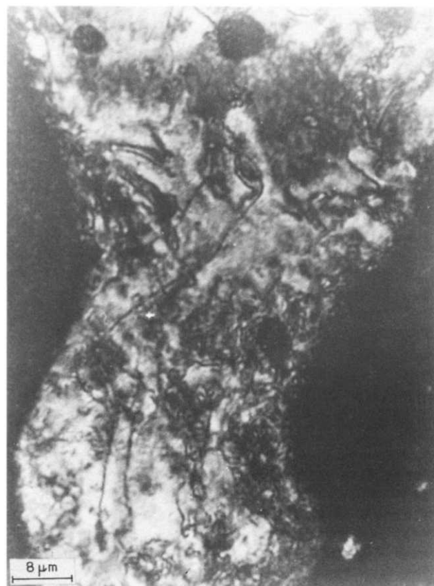
Figure 17 The effect of magnetic field. Field of 7 kGauss applied perpendicular to surface of glass slide. 'Thick section' viewed between crossed polaroids
